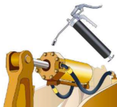
Bucket control cylinder.
